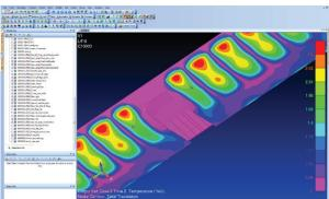
highest stresses, quickly showing where the failures are in the laminate or sandwich structure. "Scripts such as these save time and, equally importantly, help ensure the accuracy of the analyses," says Piller.
